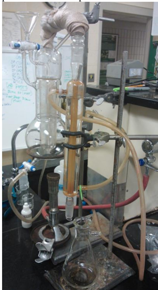
Fig 1. Markham still. The upper valve (top left corner of the picture) is at the start OPEN to the outer column. The lower valve (mid left, just next to the head of the Bunsen burner in the picture) is CLOSED. Outer column is filled with distilled water. The upper valve is then turned to OPEN for the inner column (thus CLOSED for the outer column) to pour in the grape juice sample.
